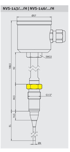
Advice for NVS-143/.../H Tighten the sensor only at the lower, marked in yellow spanner flat (BE = 22 mm)!
